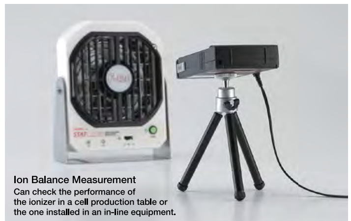
Ion Balance Plate Mount the enclosed plate to measure ion balance.
