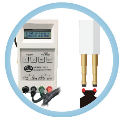
Total inspection by TREK surface resistance meter
