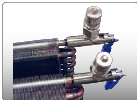
Helium Leak Test on Heat Exchangers
