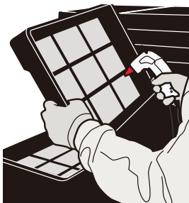
Dust removal from plastic trays
