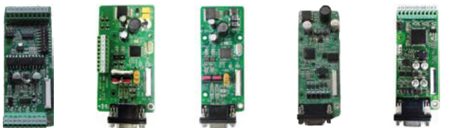
MD38PGMD: TTL differential or HTL (A/B/Z) encoder MD38PG4D: Resolver MD38PG4: Resolver ES510-PG-CT1: Serial encoder MD520-PG-S1: Sin/Cos encoder
