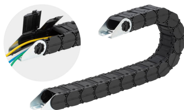
SPO series Low Abrasion, Low Noise, Full-covered Open-Close Flap Type Inner Width : 75, 100, 125, 150 [mm] Inner Height : 45, 55 [mm] Applicable Diameter : 36, 44 [mm]
